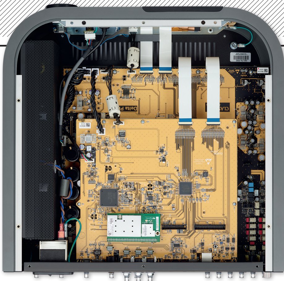
ABOVE: Delta PRE has linear PSUs [under gold-plated copper PCB] and screened switchmode supply [far left] for the digital and control circuits, including the wireless network module [green, bottom]. Large chip is main microcontroller/USB interface with AK4497 DACs and balanced o/p on lower PCB
