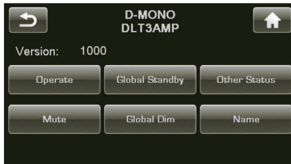
The model, name and firmware version number will be displayed on the CAN-Bus page of the targeted unit.
