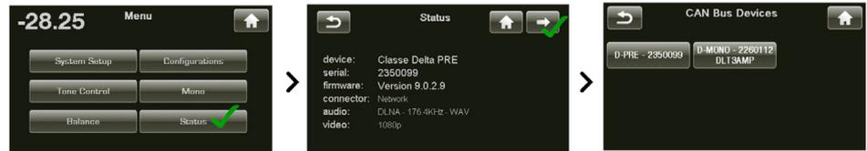
Selecting a unit on the CAN-Bus devices screen identifies it as the **target unit**. The front panel LED(s) or meter light of the target unit will start flashing (unless you choose the unit that you are using to access CAN-Bus).
