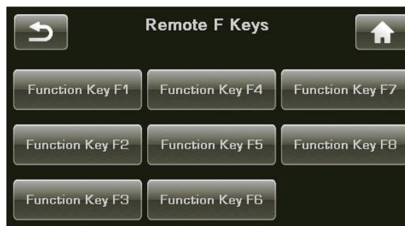
The remote control **F1** to **F8** buttons correspond to the Function Keys displayed on the touchscreen. Select the **Function Key** that you would like to assign, then scroll through the list and choose the specific function you want that **Fkey** to perform.
